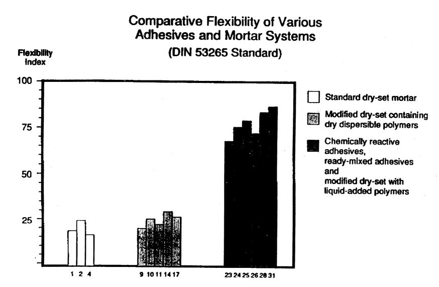
Comparative Flexibility of Various Adhesives and Mortar Systems (UEAtc Directive)
