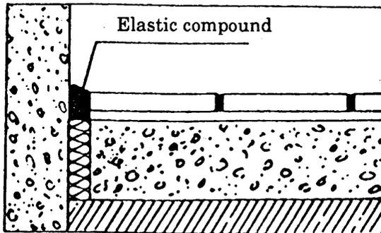
**TILE INSTALLATION IN PAVEMENTS OF HEAVY TRAFFIC
