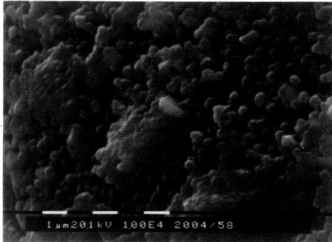
Figure 14.- Porous single-fired opaque glaze.
