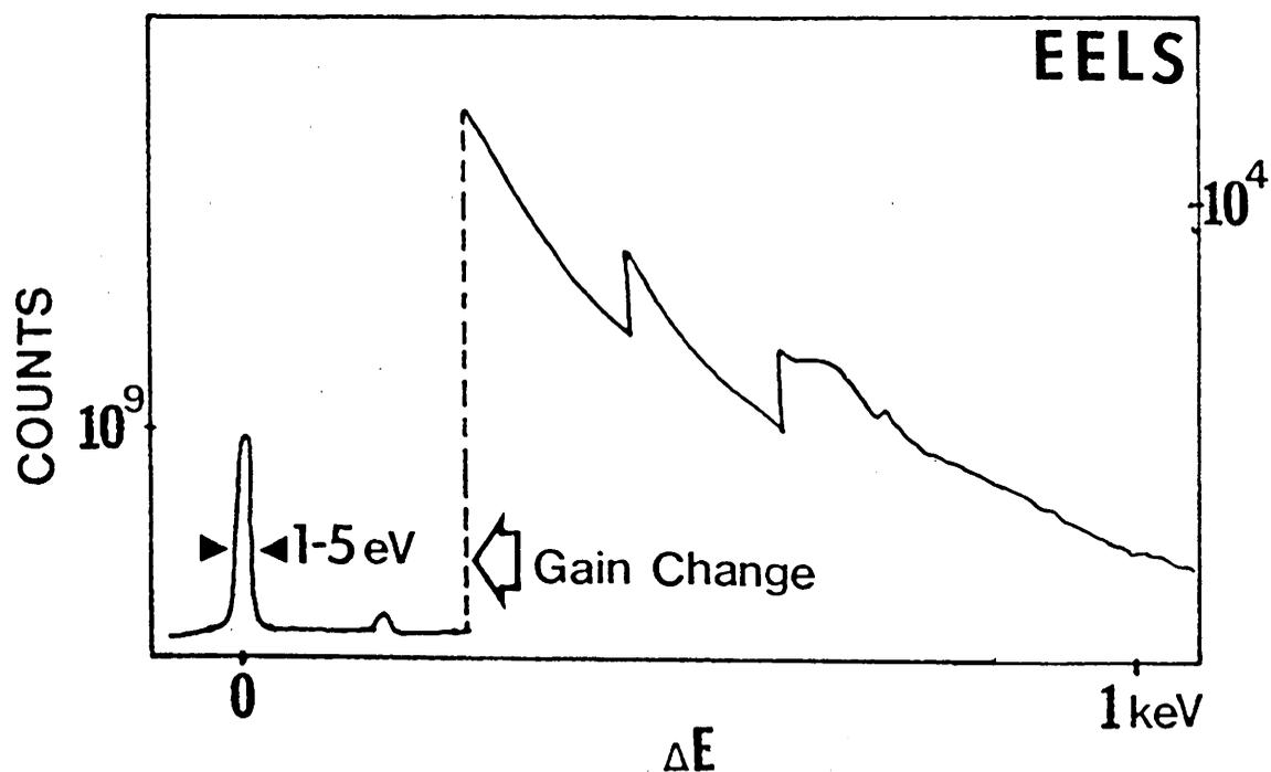
Fig. 4 Representative Model of EELS type of spectrum that is obtained from Transmission Electron Microscope.
