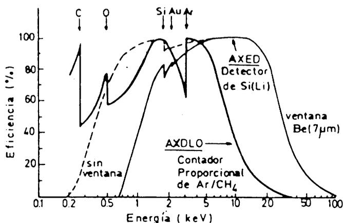
Fig. 2 Efficiency curves for different types of detectors used in MARX.
