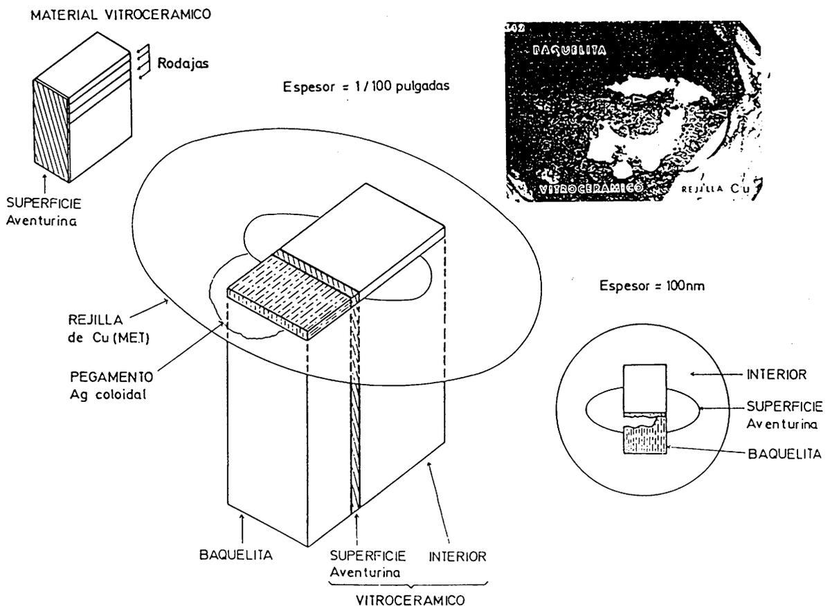
Figure 5. Diagram of transverse section obtained for the analytical electron microscopy study of both vitreous ceramic materials with a reflecting surface and aventurine effect, and the glaze-support interphase of ceramic paving and tiling.
