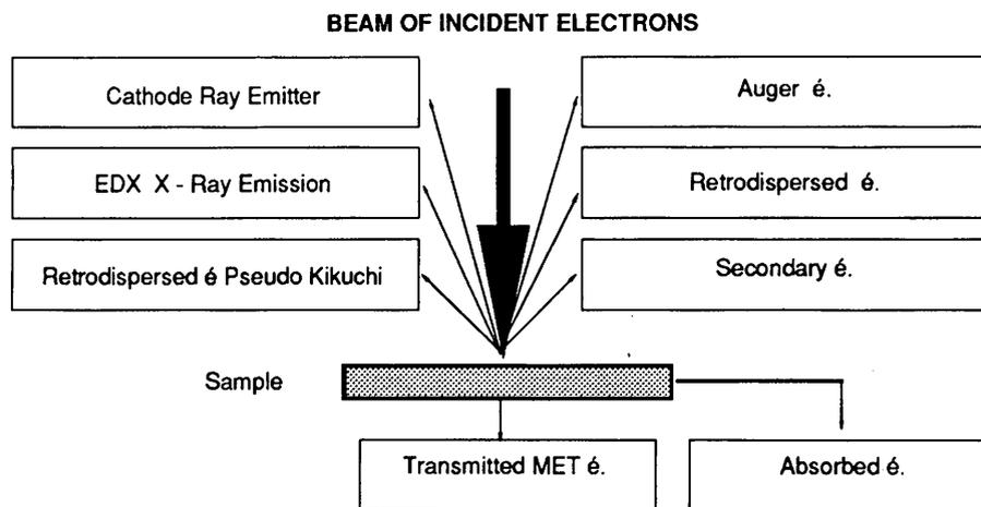
Fig. 1 - Signals that are observed in a scanning electron microscope when an electron beam is incident on the fractured surface of a ceramic material or glass.
