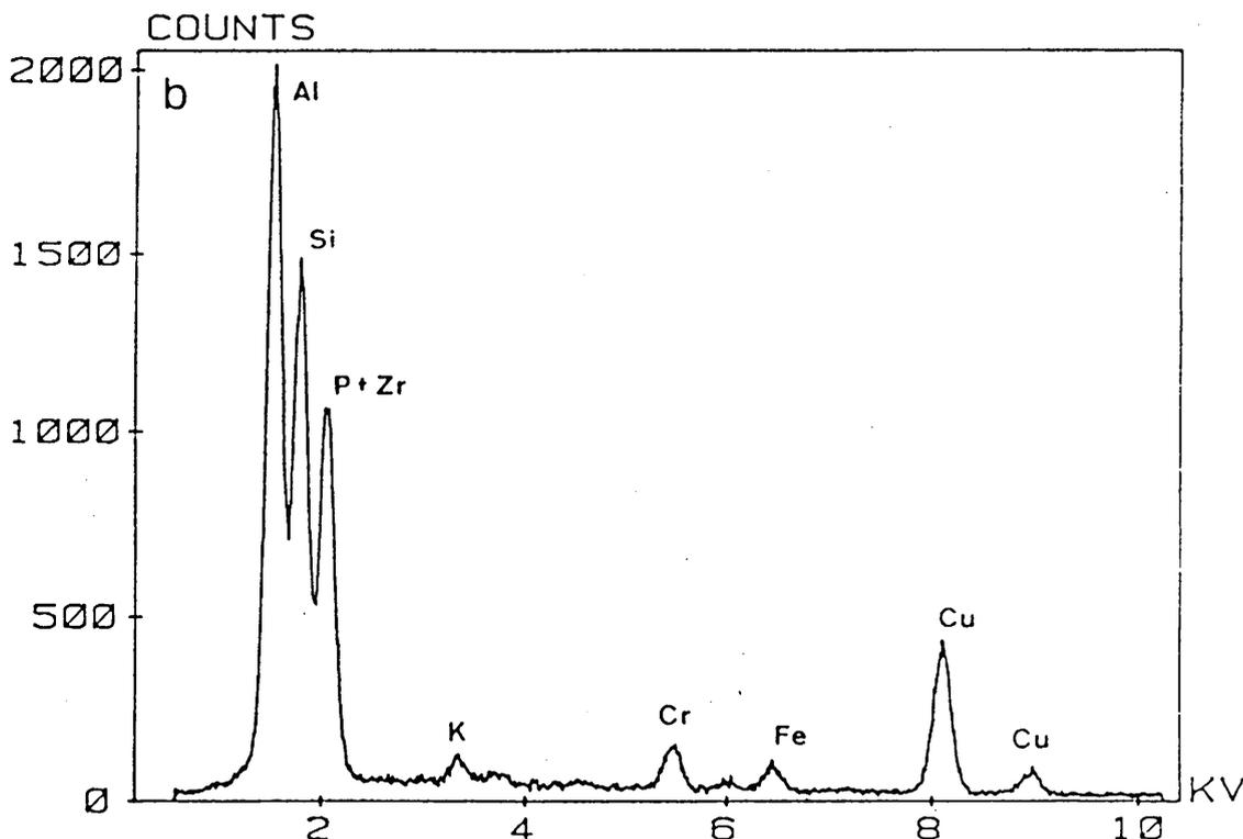
Fig. 3 - Average EDX spectrum obtained from a vitreous ceramic material with a reflective surface and an aventurine effect.
