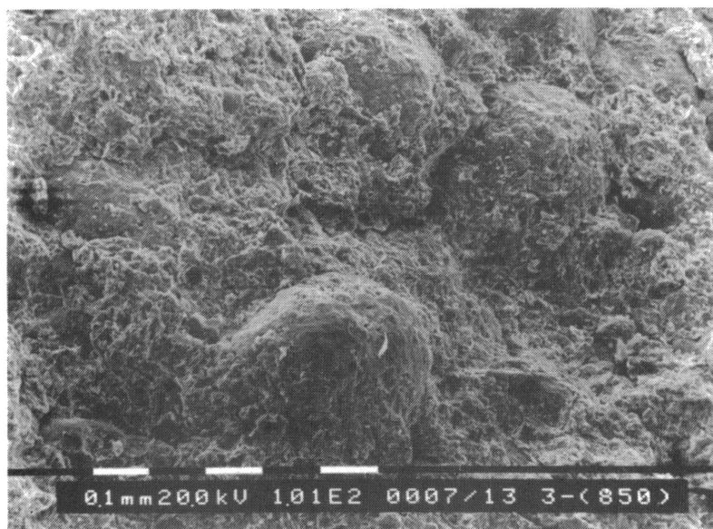
Figure 13. Microstructure of the pressed piece a X_P=0.018 kg water/kg d.s. and P=300 kg/cm 2 ; magnified 101 times.
