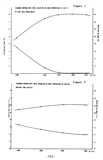
Owing to this high firing contraction, variations of porosity in the raw do on the other hand have a great effect on piece size, so that a variation of bulk density of 0.05 g/cm3 leads to a variation of firing contraction of 0.07-0.09%, almost double that of a vitrified paving tile.
