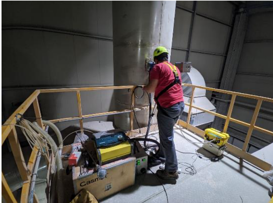
Figure 1. Monitoring of the spray dryer (flow, temperature, and humidity)
