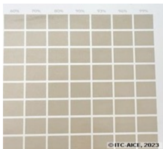
Figure 1. First screen-printing ink composition developed valorizing the by-products obtained through LIFE REPLAY implementation.
