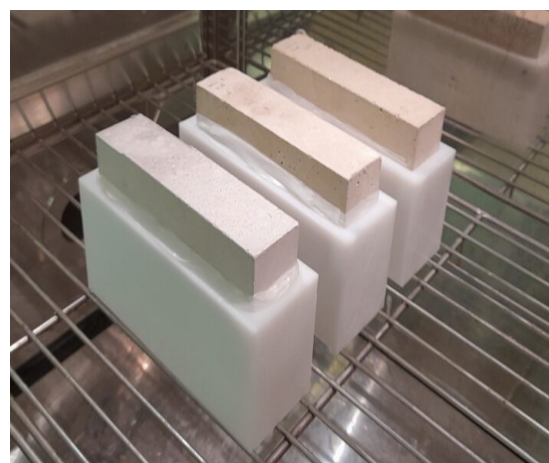
Figure 4: Left: Diagram of the experimental set-up. Right: Test specimens left in the climate chamber for 15 days.
