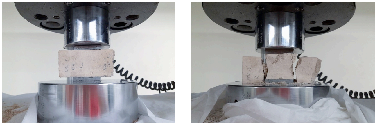
Figure 3: Left: Experimental set-up. Right: Broken test specimen.
