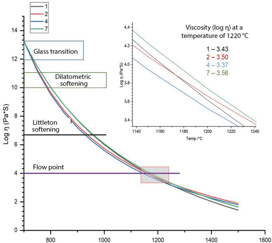
**Figure 5.** Viscosity in the glazes studied in Phase 2 using the Vogel-Fulcher-Tammann (VFT) formula.
