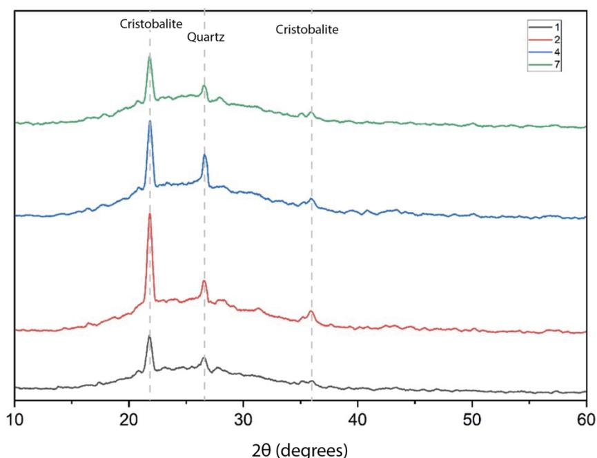
**Figure 6.** X-ray diffraction results for the formulations studied in Phase 2.
