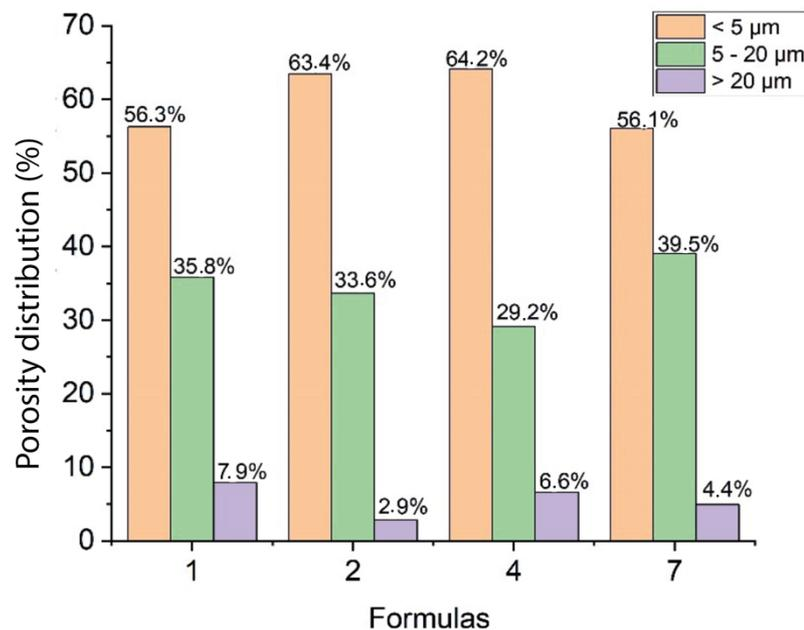
**Figure 7.** Percentage and average diameter of surface pores in the glazes in Phase 2.
