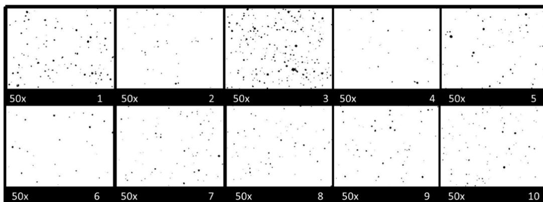
**Figure 2.** Testing Surface porosity with Image J software.
