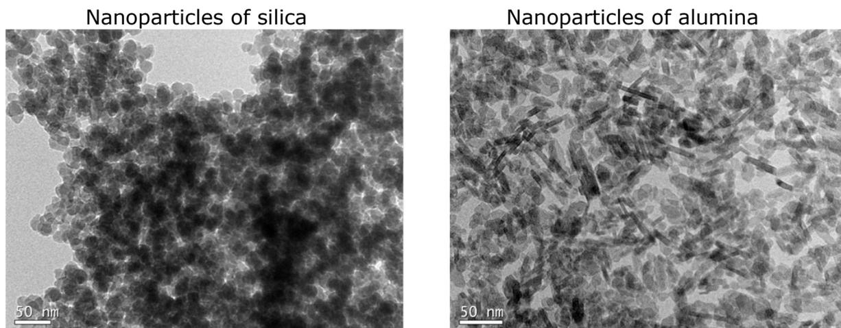
**Figure 1.** Transmission electron microscopy of the silica and alumina nanoparticles.
