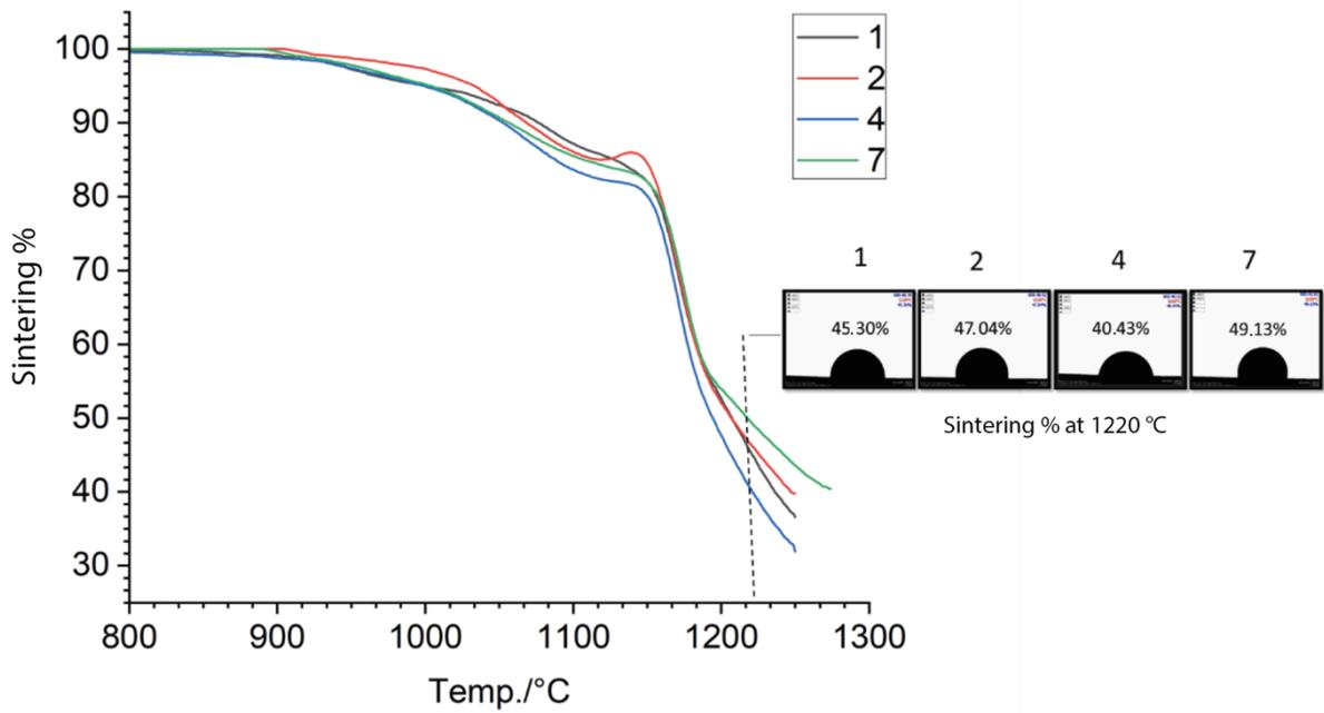
**Figure 4.** Sintering curve versus temperature in the formulations selected for Phase 2.
