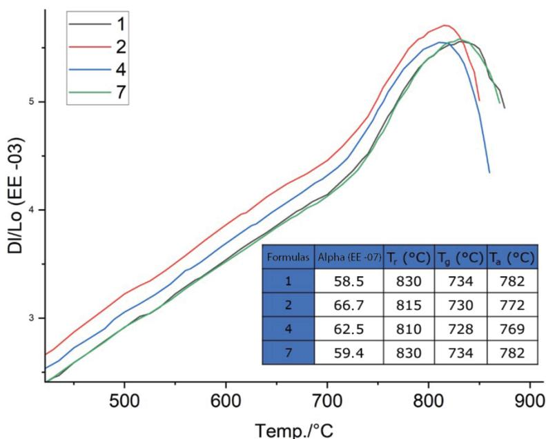
**Figure 3.** Results of the dilatometric curves for the formulations studied in Phase 2.
