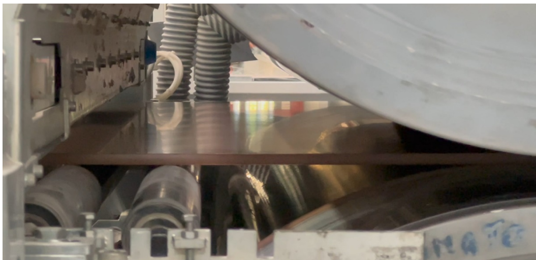
Figure 10 - compacted slab exiting the machine
