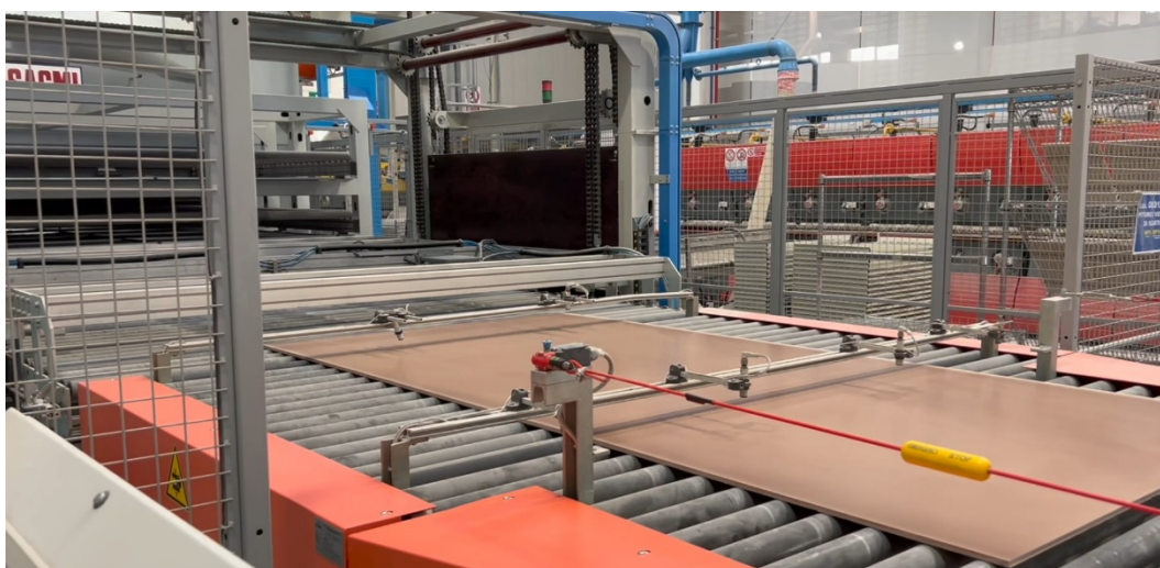
Figure 12 - slab at the dryer inlet
