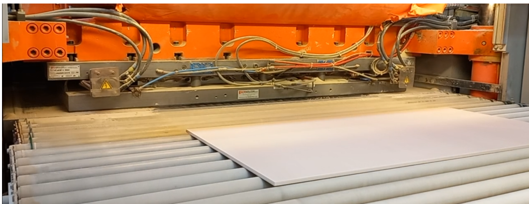
Figure 16 – 600x1200 mm pressed tile
