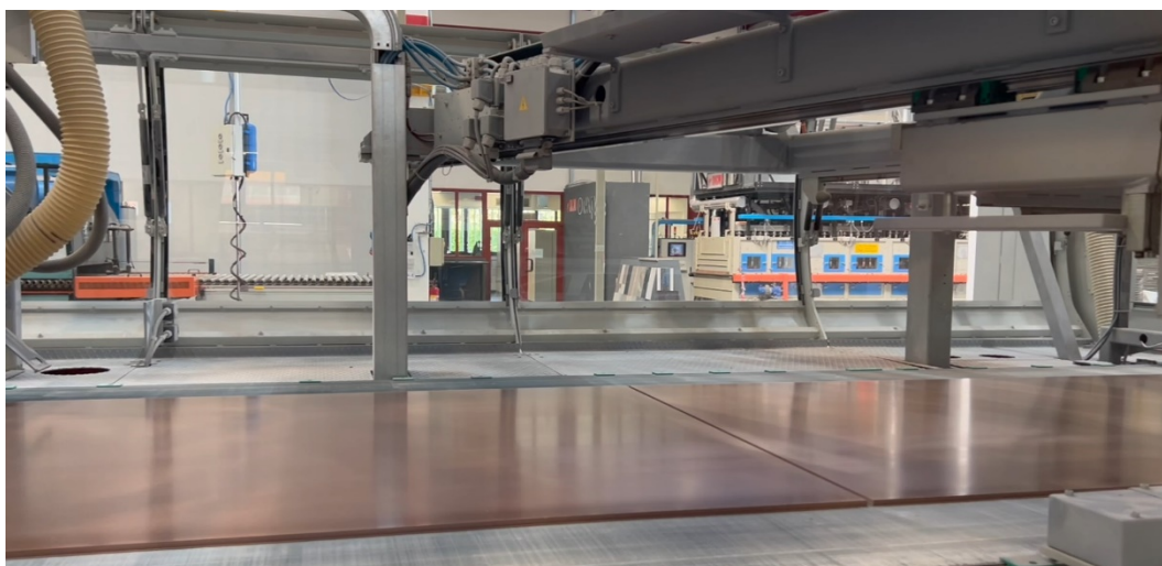
Figure 11 - slab on the cutting belt
