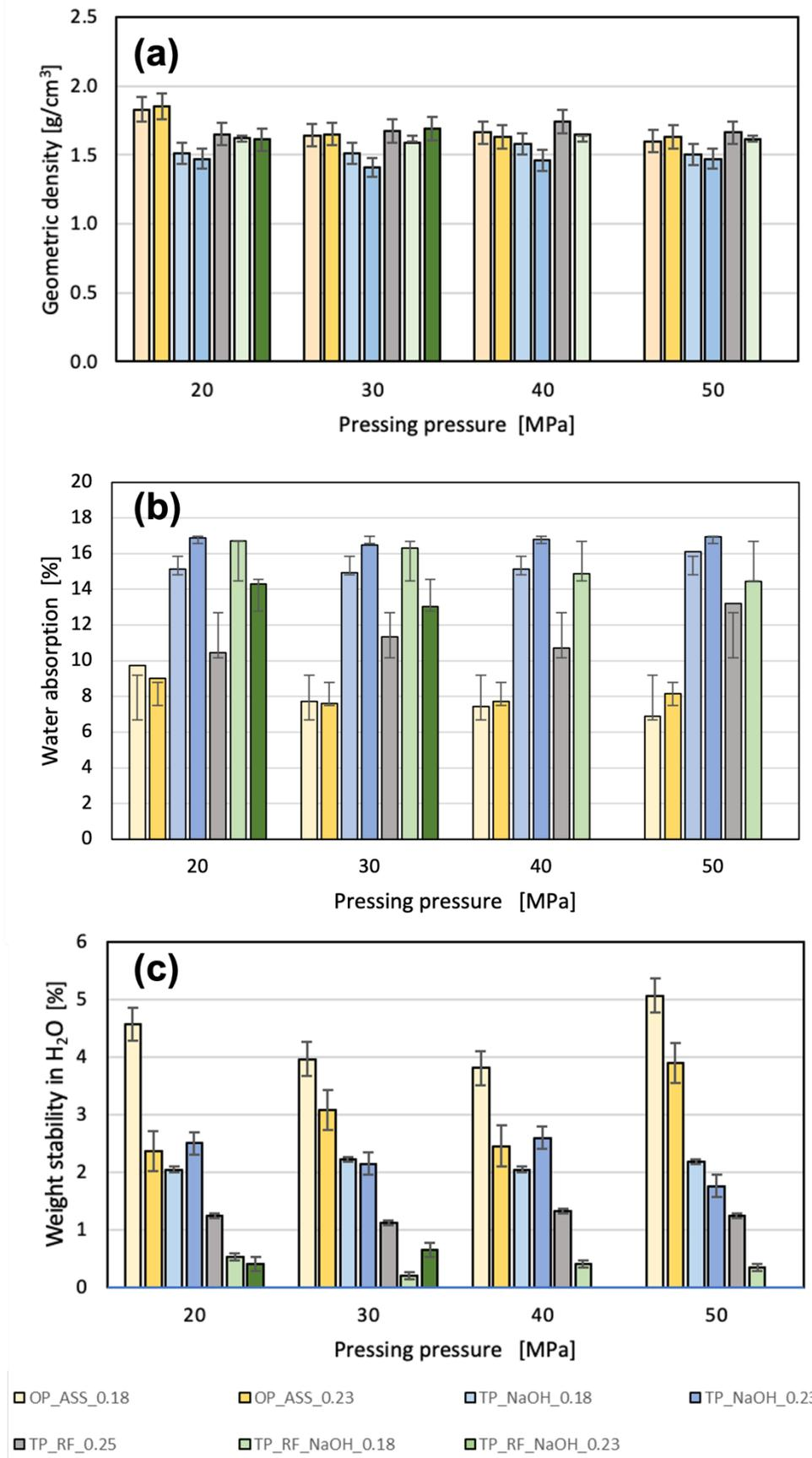
**Figure 1:** Geometric density (a), water absorption (b) and weight loss (c) of all the samples cured at room temperature for 7 days.
