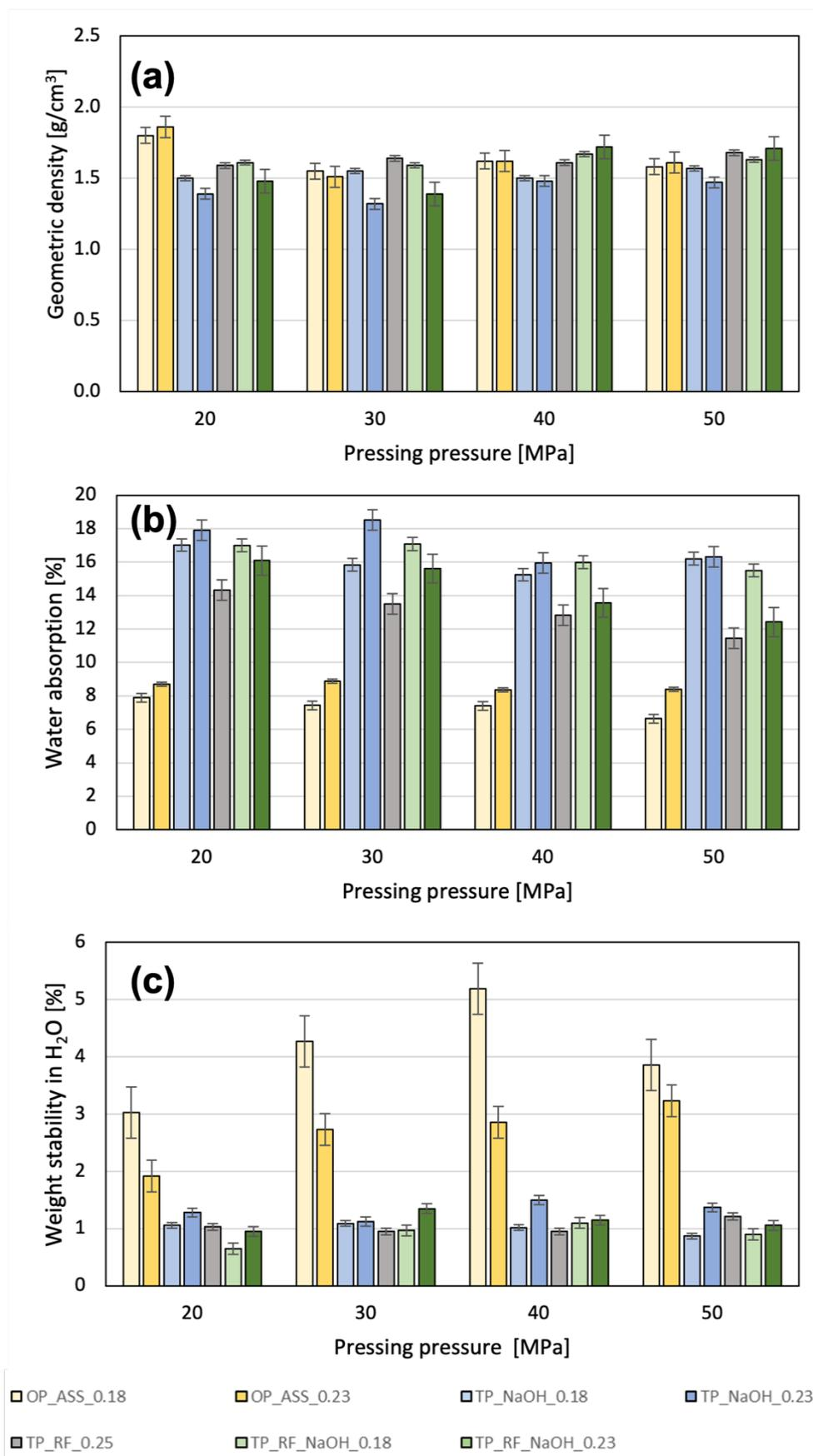
**Figure 3:** Geometric density(a), water absorption (b) and weight loss (c) of all the samples cured at 70 °C for 24h.
