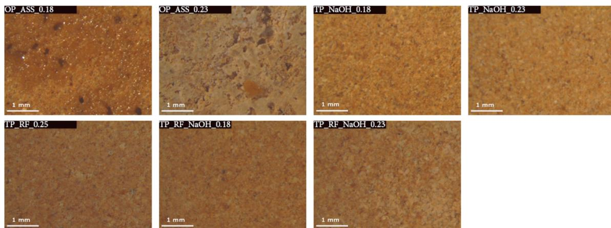
**Figure 4:** Microstructural observations performed by optical microscopy of all the geopolymers pressed at 20 MPa and cured at 50 °C.
