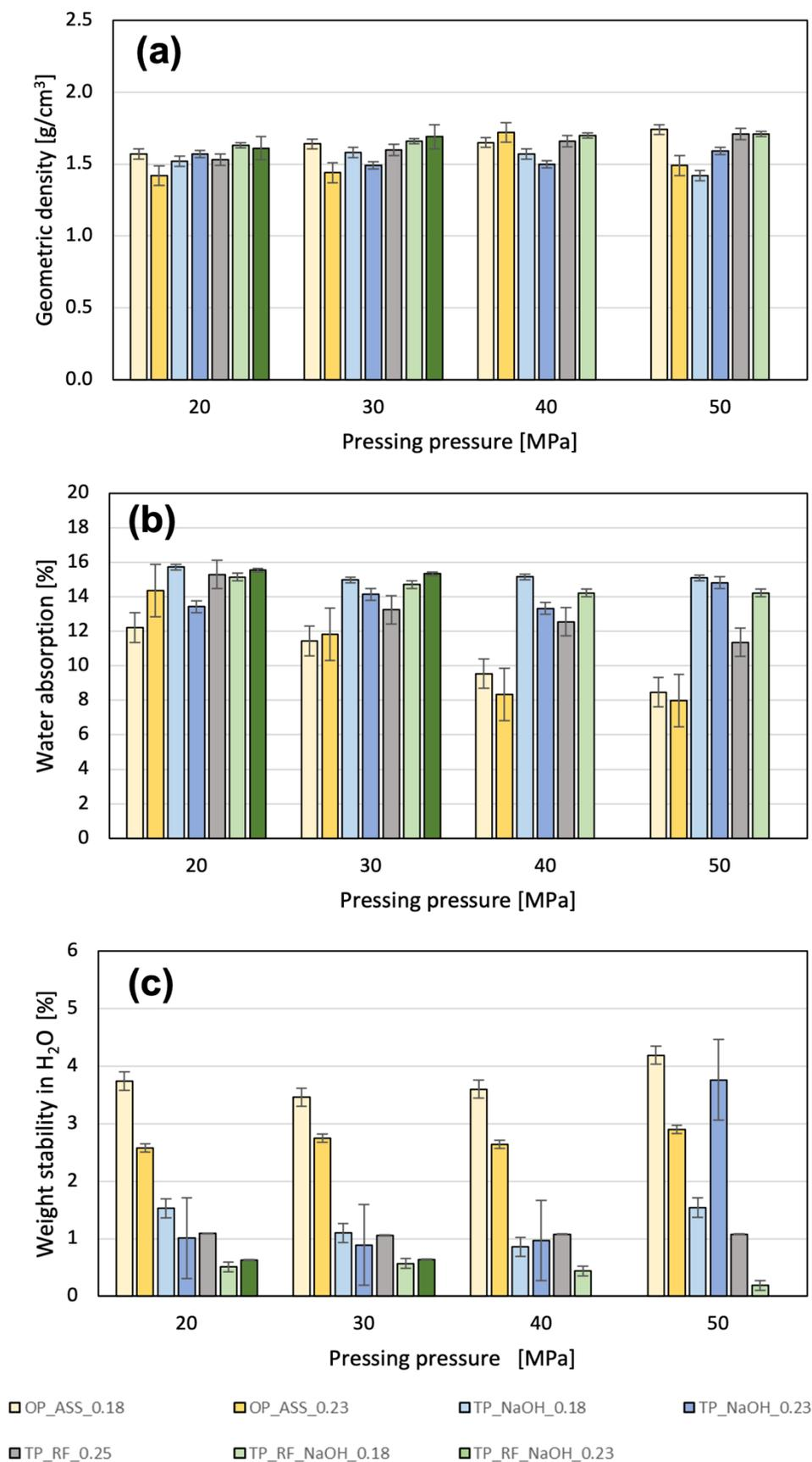
**Figure 2:** Geometric density(a), water absorption (b) and weight loss (c) of all the samples cured at 50 °C for 24h.
