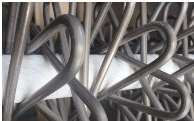
Fig. 8 – Close-up of the elements that make up the electric heater.
