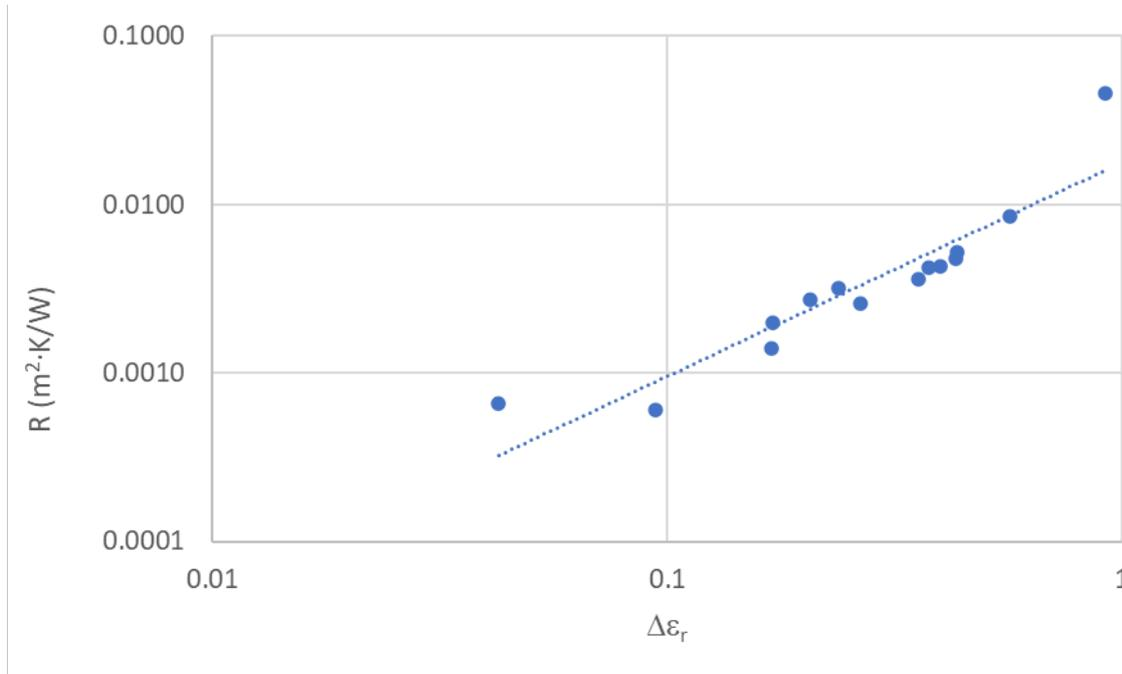
**Figure 6.** Correlation between thermal contact resistance and relative effusivity variation ( $R=0.0178 \cdot \Delta\epsilon_r^{1.27}$ ,  $r^2=0.8$ )
