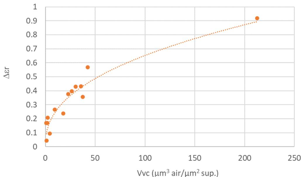
**Figure 7.** Influence of the average thickness of trapped air on the relative change in effusivity ( $\Delta\varepsilon_r = 0.0947 \cdot V_{vc}^{0.419}$ ,  $r^2 = 0.92$ )
