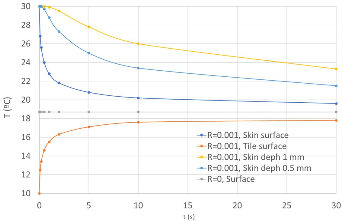
**Figure 4.** Simulation of tile and skin thermal behaviour.  $R$  in  $m^2K/W$  units.
