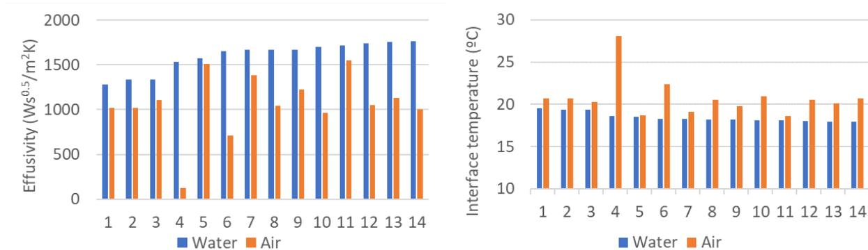
**Figure 5.** Actual and effective effusivity of the sample set used (left). Contact temperatures (right).
