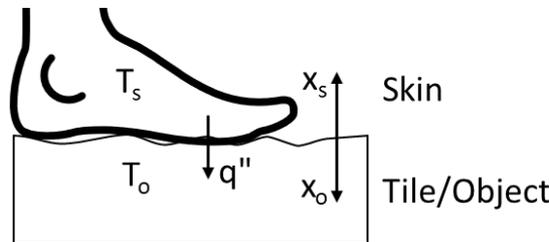
**Figure 1.** Heat transfer process scheme between the sole and the tile.
