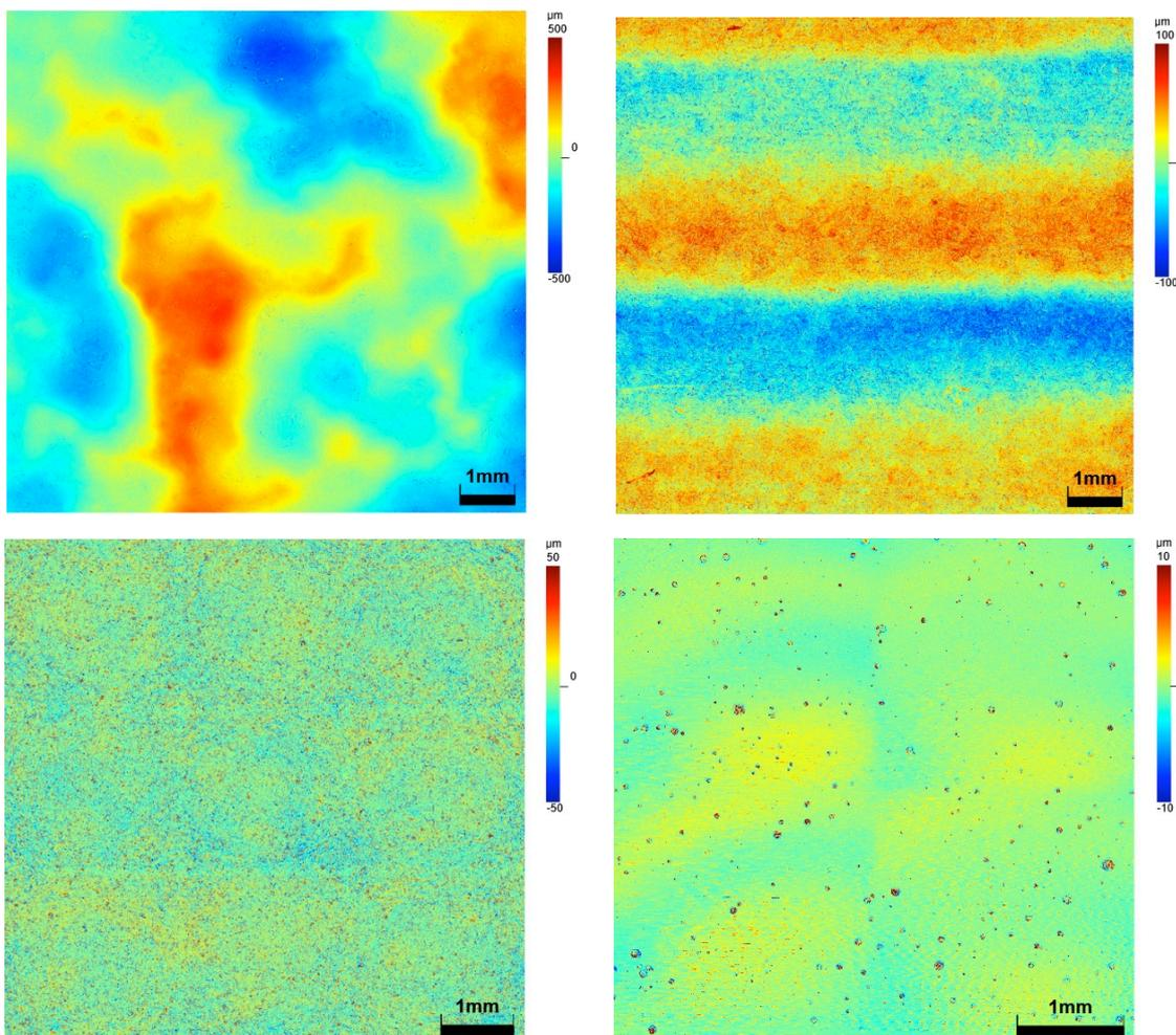
**Figure 2.** Topographies of samples 4 (top left, press relief,  $\pm 500\mu\text{m}$ ), 6 (top right, glaze line relief,  $\pm 100\mu\text{m}$ ), 3 (bottom left, matt glaze,  $\pm 50\mu\text{m}$ ) and 5 (bottom right, polished glaze,  $\pm 10\mu\text{m}$ ).
