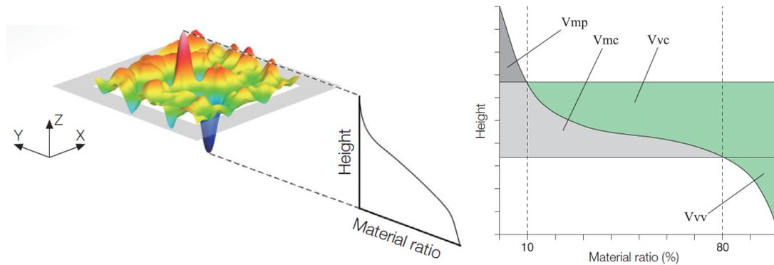
**Figure 3.** Calculation of the material curve from the topographic data (left). Calculation of the Core void volume ( $V_{vc}$ ) from the material curve (right).
