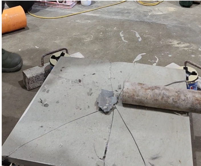
Photo 5. Tile fractured on pedestals, reinforced with a fiberglass matting adhered with cementitious adhesive. Load used to break the tile was a 10kg steel weight with a diameter of 60mm.
