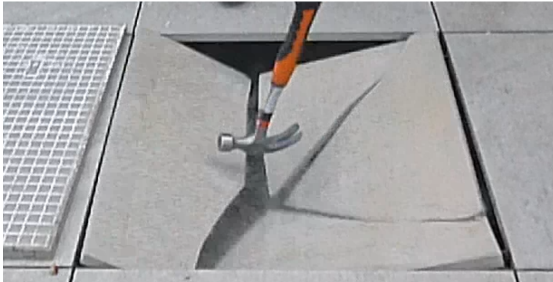
Photo 4. Screen shot from a video where I was able to break a 20mm porcelain tile dropping a 906g (2lbs) claw hammer from 600mm).
