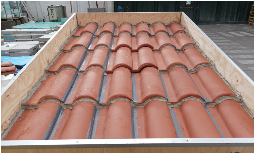
Figure 4: Unsealed elements of the assembly.
