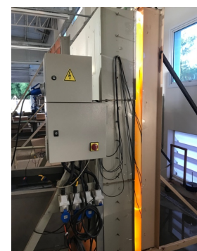
Figure 8– Thermal shock chamber with the prototypes.
