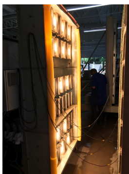
Figure 8– Thermal shock chamber with the prototypes.
