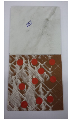
Tile with simulation of 25% setting failure – 75% filling of under tile
