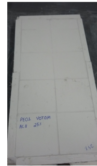
Prototype covered with porcelain tiles and ACIII mortar with 25% setting failure and with elastomeric grout – with restriction
