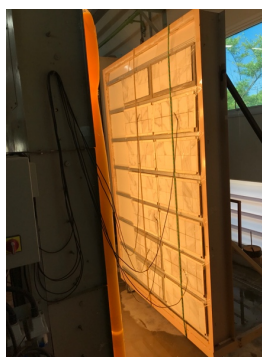
Figure 8– Thermal shock chamber with the prototypes.
