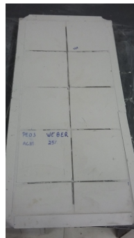
Prototype covered with porcelain tiles and ACIII mortar with 25% setting failure and with elastomeric grout
