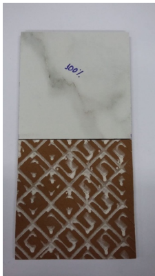
Tile without setting failure simulation – 100% filling of under tile
