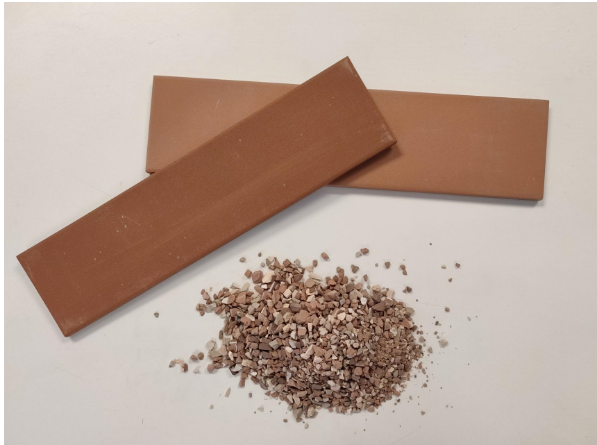
Figure 2. Ceramic tile bodies manufactured with 40% fired tile scrap incorporated into the composition. Source: ITC-AICE
