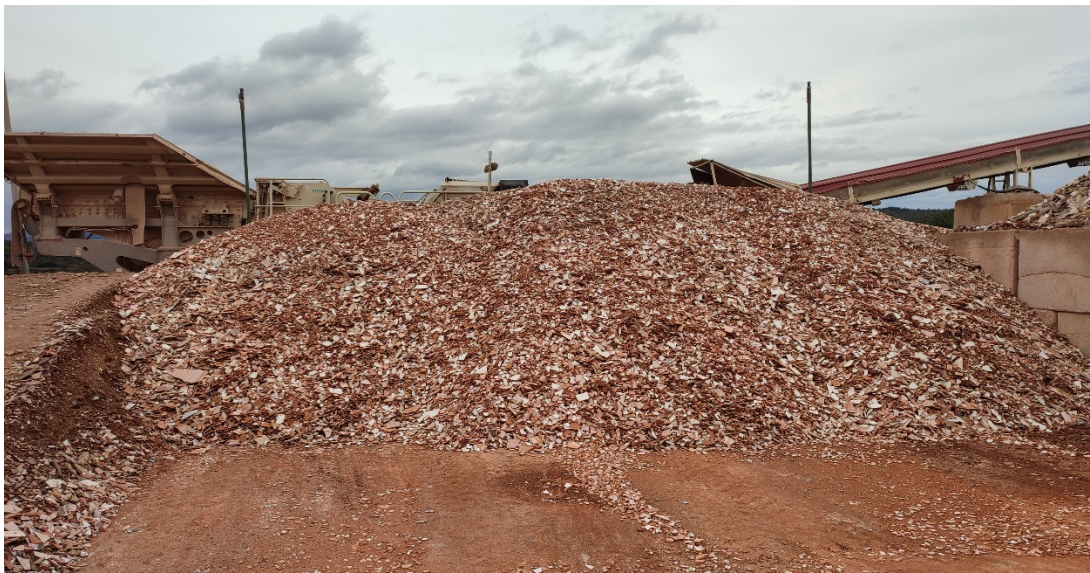
Figure 1. Fired red-body tile scrap at the ECOVILAR S.L. waste management site. Source: ITC-AICE
