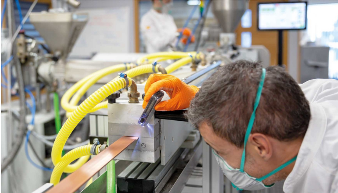
Figure 4. Obtaining PVC profiles by incorporating fired red-body tile scrap as mineral filler. (Source: SAXUN - Giménez Ganga)
