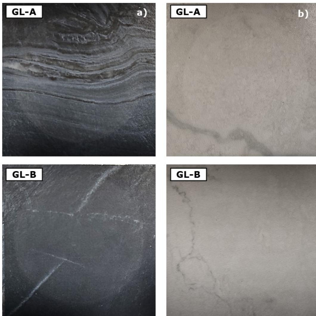
**Figure 1:** Abraded areas of GL-A and GL-B glazed tiles. a) Abraded area visible after 600 cycles, b) abraded area after 12000 cycles
