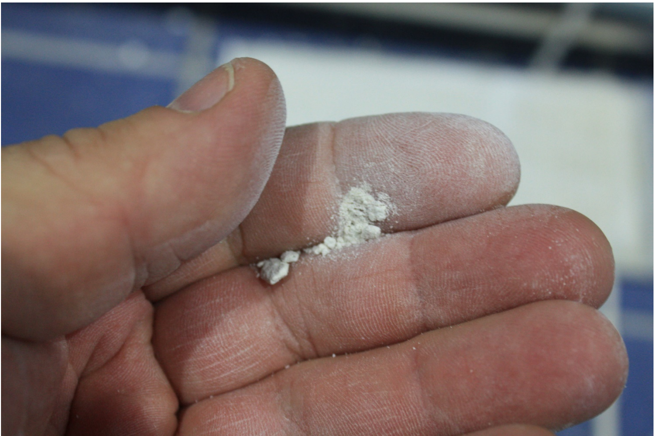
Photograph 6- shows adhesive crumbling into a powder.
