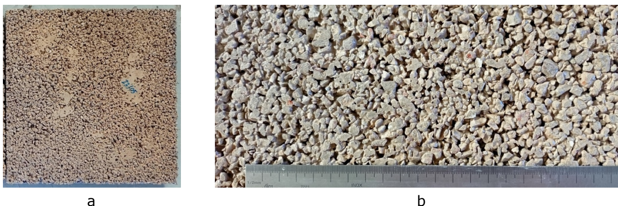
Figure 3. Porous concrete pavers with ceramic tile waste: a) General view; b) Close-up.
