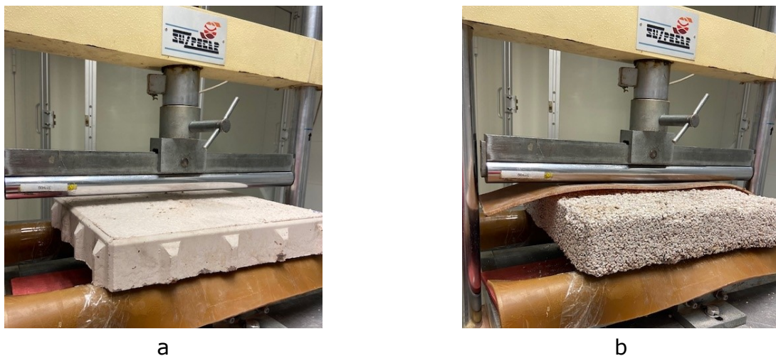
Figure 8. Determination of bending strength of pavers produced by the precast firm: a) Compact; b) Porous.
