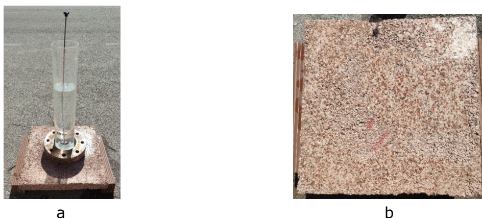
Figure 4. Determination of permeability in porous pavers; (a) Permeability test; (b) Rough-ground face of the porous paver.
