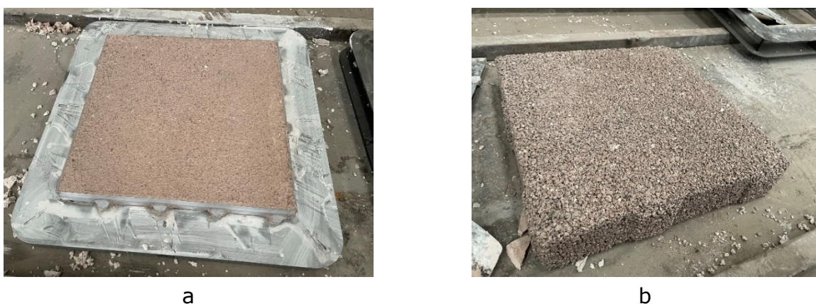
Figure 7. Development of the pavers at the precast firm: a) compact, in mould; b) porous, demoulded.
