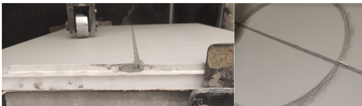
Figure 6: Left: Detail of the test setup. Right: Example of non-compliance with acceptance criteria
