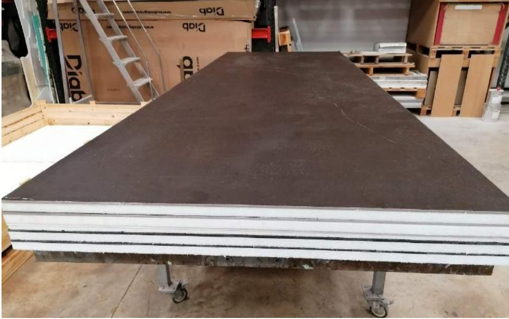
Figure 14. Photos of ceramic sandwich slabs for drywall cladding.
