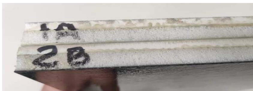
Figure 12. Test specimens subjected to the hot / cold test.
