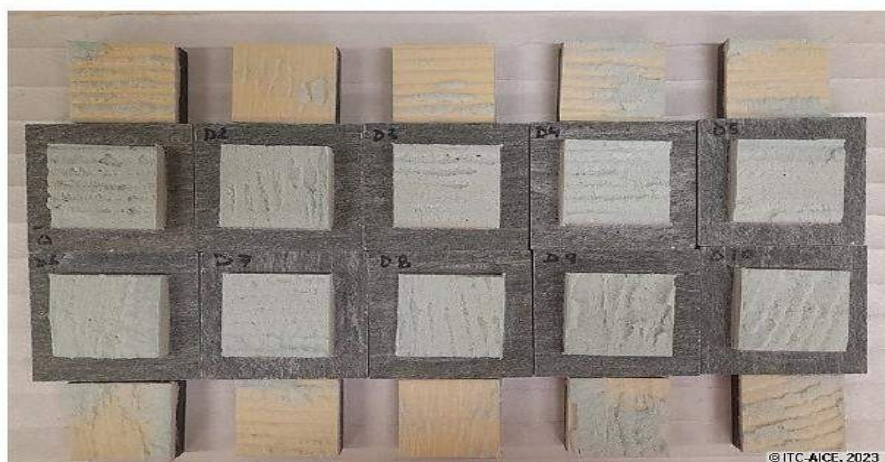
Figure 09. Photo of the adhesion strength test specimens.
