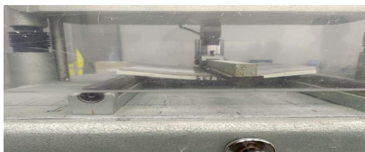
Figure 04. Photo of ceramic sandwich bending test.
