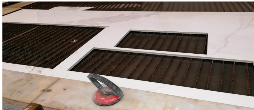
Figure 15. Photo of a ceramic sandwich cut with a five-axis water jet machine.
