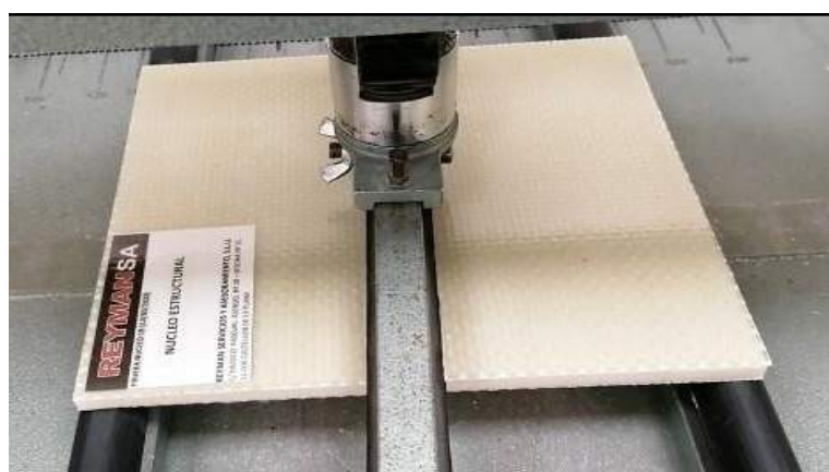
Figure 10. Photo of the bending test on the raised floor sandwich.
