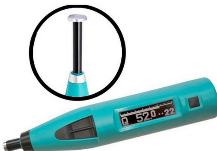
Figure 5. A "low impact" Schmidt Hammer with mushroom head (circled) for testing thinner more brittle surfaces such as ceramic tiles. (NOTE: Some surfaces such as thin ceramics and mosaics may still be damaged by the mushroom head).
