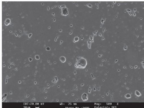
Figure 13. Micrograph (SEM/EDX) of the polished surface of sample P4 fired at 1190.
