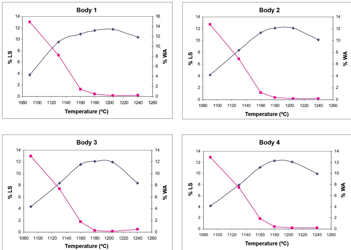
Figures 5-8. Vitrification diagrams of the porcelain tile compositions formed by pressing.
